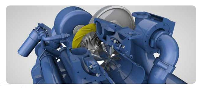
Turbo compressors are the type of compressors that provide kinetic energy to the air or gases by the centrifugal force generated by the impellers and convert this kinetic energy into pressure energy in the diffuser by reducing the air flow path. Pressurized air is cooled before entering the next stage with high performance coolers. This results in higher productivity.
