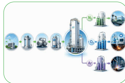
Air Separation Unit
