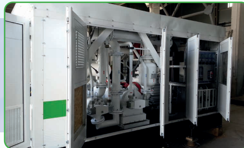
High Pressure Bio-CNG Compressors
